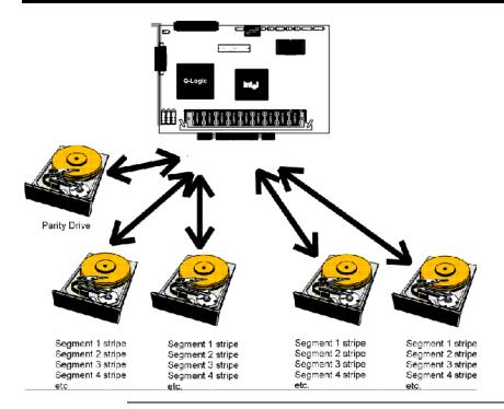
RAID 5 vs RAID 3 You may find that RAID 5 is preferable to RAID 3, even for applications characterized by sequential reads and writes, because MegaRAID Express 500 has very robust caching algorithms.
